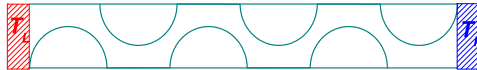
Fig. 2. The geometry of the Lorentz gas channel model. The two heat reservoirs at temperatures T_L and T_R are indicated.
